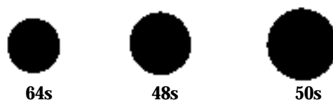
Figure 2. Relative diameters of some of the English or Spinning Count wool grades (x 500 magnification).
